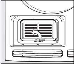
■ Turn the lever on the condenser unit upwards to the vertical position.
